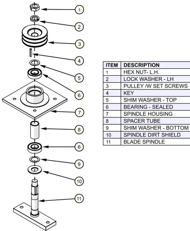
If bearings are being changed, be sure to check bearing spacer for wear. If wear is noticed, insert new spacer. This is critical because if spacer is short by only .010", the top bearing will start to bind and will result in premature failure.
